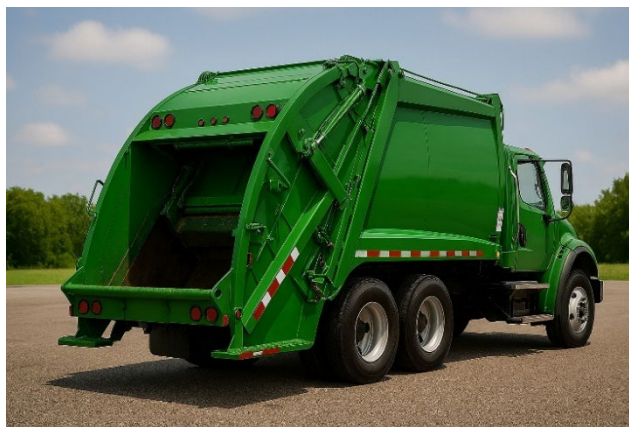
Figure 1: Illustrative Example of Rear Load Garbage Truck
